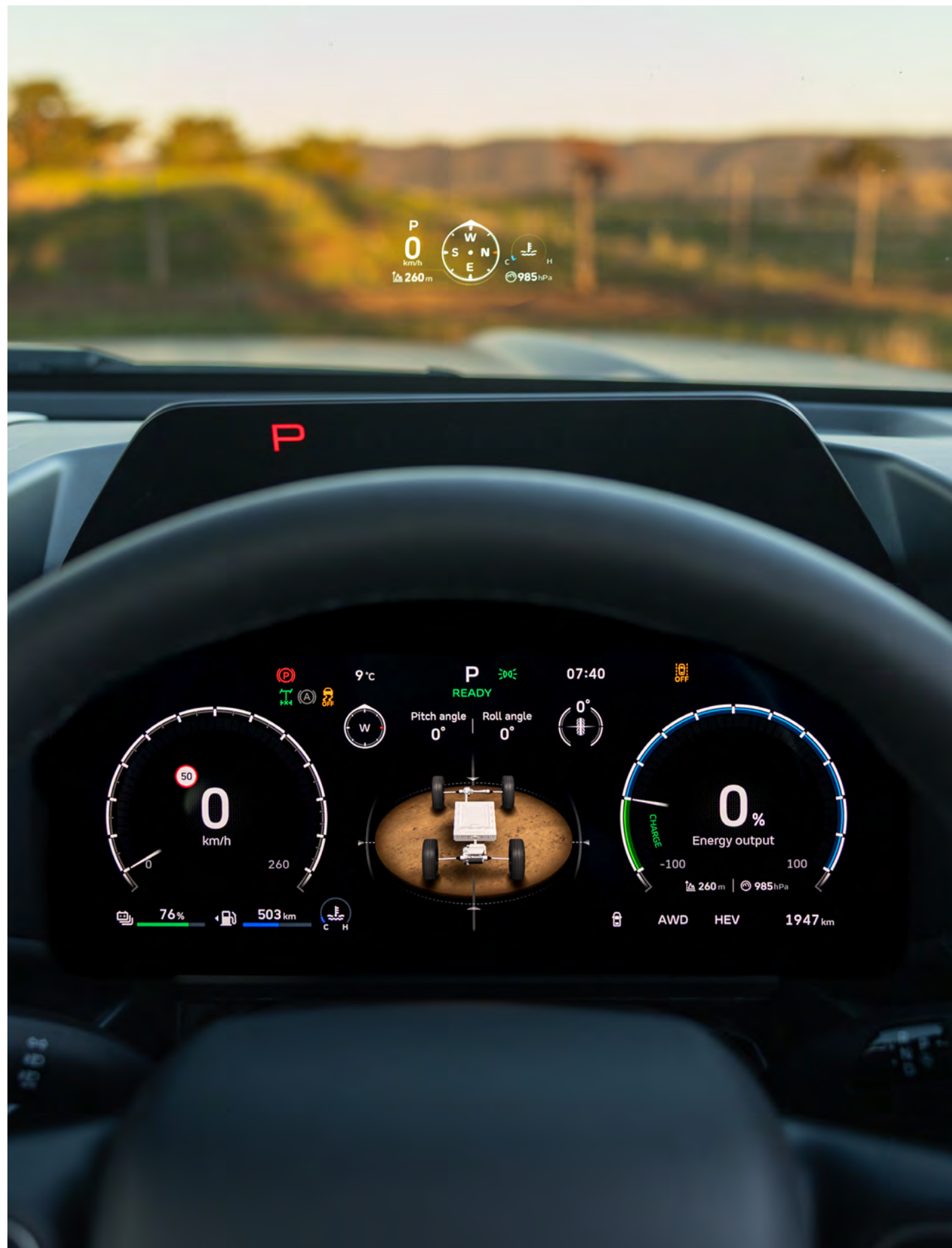
12.6" LCD Driver Display and 9" Head Up Display
